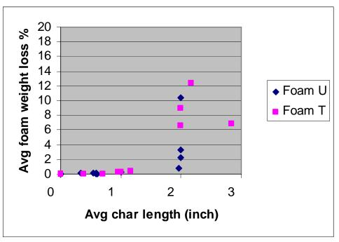
Figure 36. Char Length vs. Weight Loss – Interliner S
