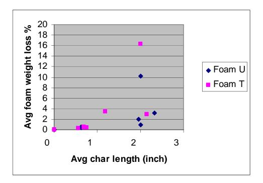
Figure 37. Char Length vs. Weight Loss – Interliner M
