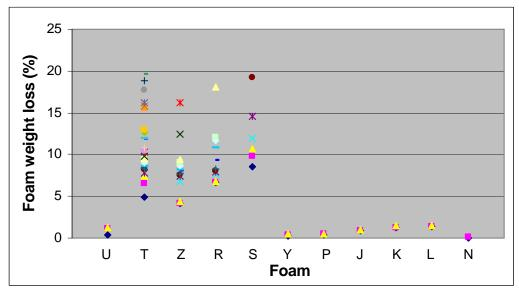
Figure 18. Foam Weight Loss of Mockups Tested with Fabric 24
