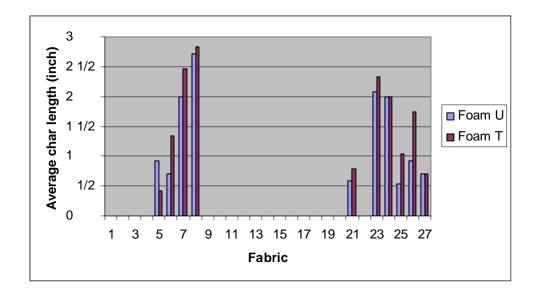
Figure 26. Char Length: Foam U vs. Foam T with Interliner V
