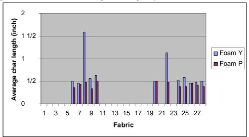
Figure 5. Average Char Length – Foam Y vs. Foam P (No Interliner)
