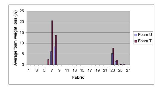
Figure 29. Weight Loss: Foam U vs. Foam T with Interliner L
