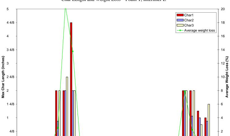
Char Length and Weight Loss – Foam T, Interliner L
