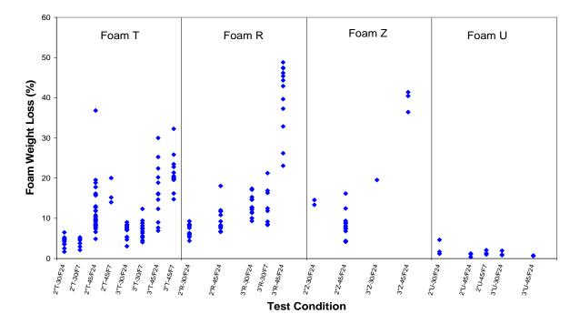
Figure 41. Smoldering Test Foam Weight Loss Data (2" vs. 3" at 30 and 45 minutes)
