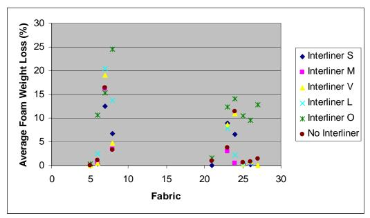
Figure 11. Foam Weight Loss – Foam T with and without Interliner
