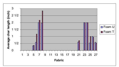
Figure 22. Char Length: Foam U vs. Foam T with Interliner S
