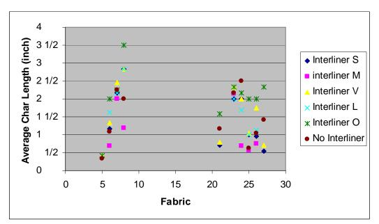
Figure 10. Char Length - Foam T with and without Interliner
