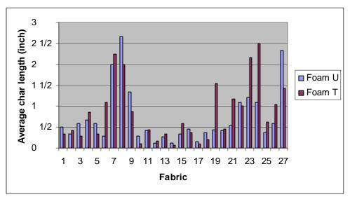
Figure 3. Char Length – Foam U vs. Foam T (No Interliner)
