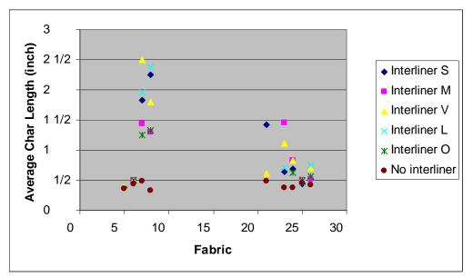
Figure 14. Char Length – Foam P with and without Interliner
