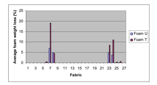
Figure 27. Weight Loss: Foam U vs. foam T with Interliner V
