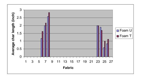
Figure 28. Char Length: Foam U vs. Foam T with Interliner L
