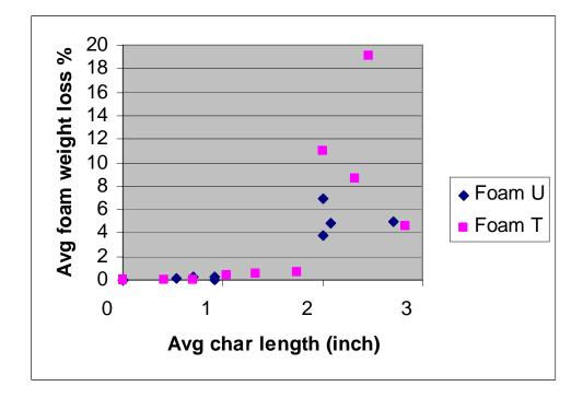
Figure 38. Char Length vs. Weight Loss – Interliner V
