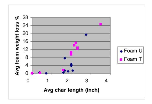
Figure 40. Char Length vs. Weight Loss – Interliner O
