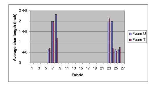
Figure 24. Char Length: Foam U vs. Foam T with Interliner M
