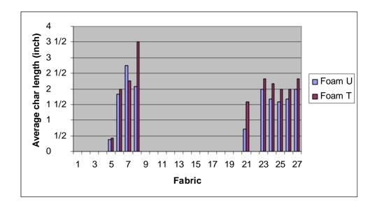
Figure 30. Char Length: Foam U vs. Foam T with Interliner O
