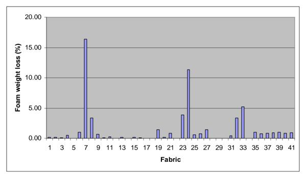
Figure 17. Foam Weight Losses of Mockups made from Foam T and all Fabrics
