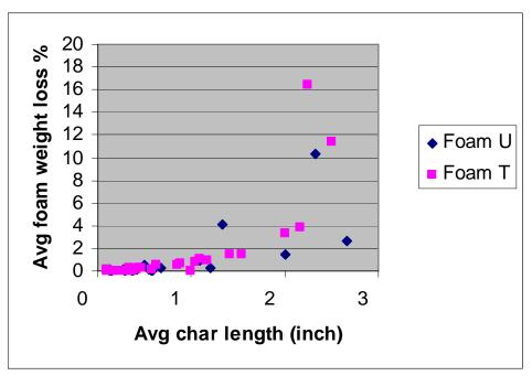
Figure 35. Char Length vs. Weight Loss - No Interliner
