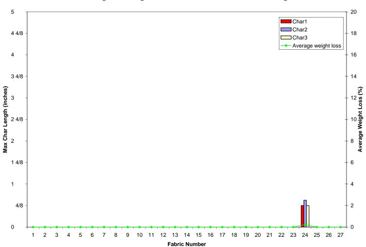
Char Length and Weight Loss – Foam T, Interliner D/UFAC Batting
