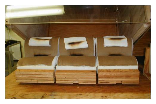
Figure 16 (a). Post Test Mockups of Fabric 24 with Foam U and UFAC Polyester Batting (top)/Interliner V (under)
