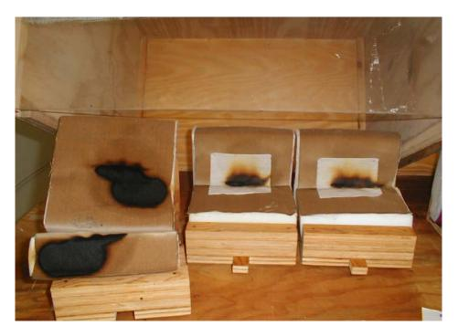
Figure 34. Post Test Mockups of Fabric 24 with Foam U and Interliner V
