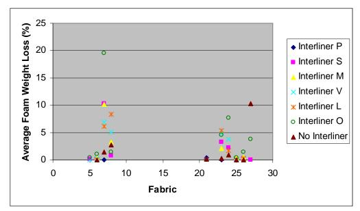
Figure 9. Foam Weight Loss - Foam U with and without Interliner
