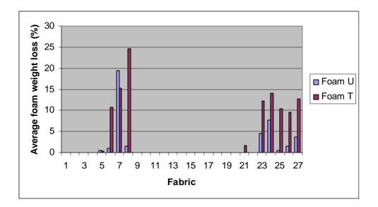
Figure 31. Weight Loss: Foam U vs. Foam T with Interliner O
