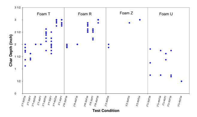
Figure 43. Smoldering Test Foam Char Depth Data
