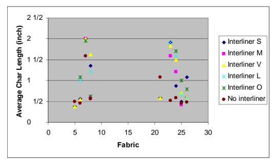
Figure 12. Char Length – Foam Y with and without Interliner
