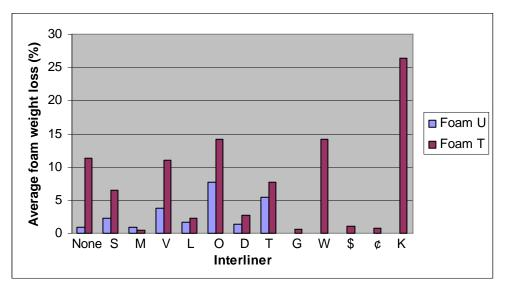
Figure 21. Comparison of Foam Weight Loss of TB117+ Cotton Velvet Fabric Tested with Different Interliners and without Interliners
