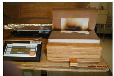
Figure 2. Post Test Mockup of Fabric 24 with Foam T
