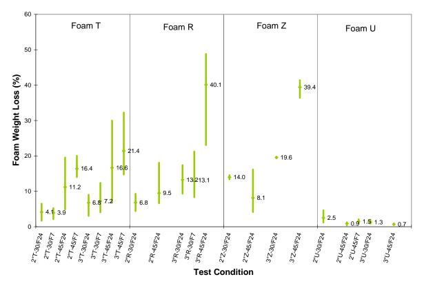
Figure 42. Smoldering Test Foam Weight Loss (High, Low, Average, 2" vs. 3" at 30 and 45 minutes)
