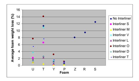
Figure 33. Comparison of Foam Weight Loss of TB117+ Cotton Velvet Fabric Tested with Different Foams and Interliners
