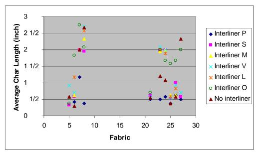
Figure 8. Char Length – Foam U with and without Interliner
