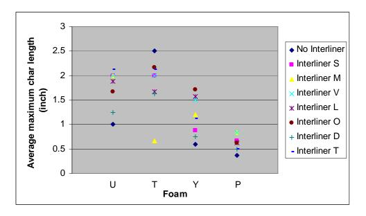
Figure 32. Comparison of Char Length of TB117+ Cotton Velvet Fabric Tested with Different Foams and Interliners
