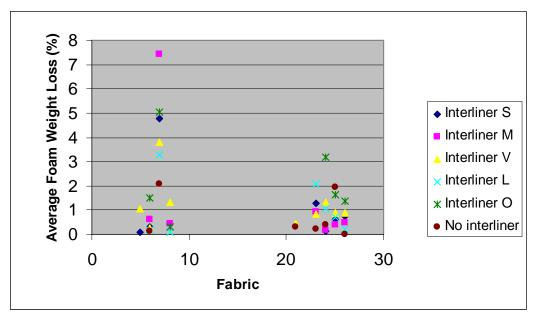
Figure 13. Foam Weight Loss – Foam Y with and without Interliner
