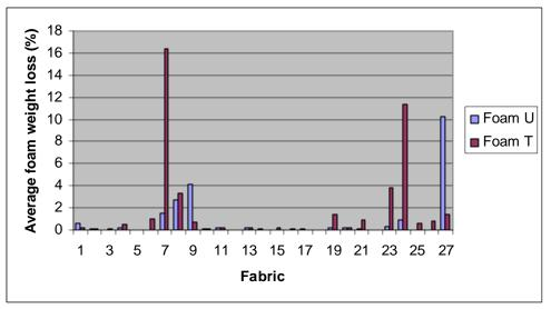
Figure 4. Foam Weight Loss - Foam U vs. Foam T (No Interliner)
