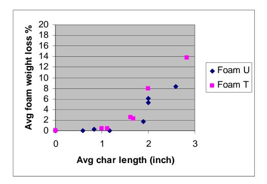
Figure 39. Char Length vs. Weight Loss – Interliner L
