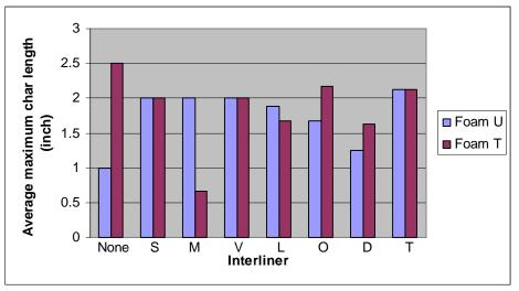
Figure 20. Comparison of Char Length of TB117+ Cotton Velvet Fabric Tested with Different Interliners and without Interliners
