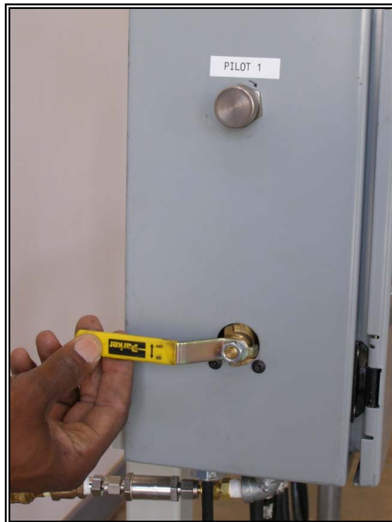
Figure 31. Step 32 Open pilot ball valves.
