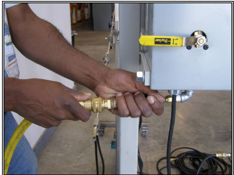
Figure 9. Step 2 Connect propane supply.
