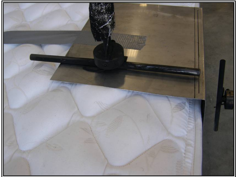
Figure 19. Step 15 Position burner head.
