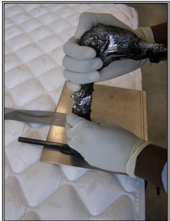
Figure 18. Step 14 Make burner face parallel to platen.
