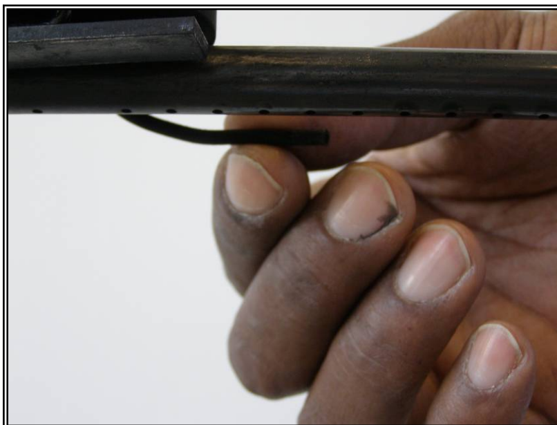
Figure 15. Step 11 Check pilot tube.
