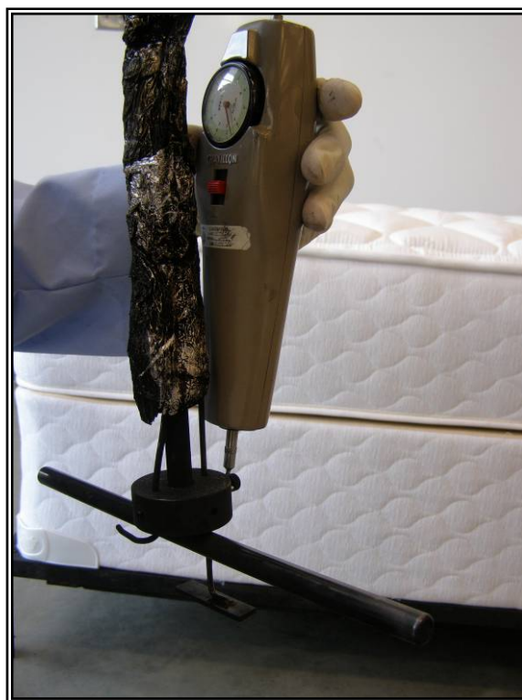
Figure 27. Step 23 Measure downward force using spring scale.
