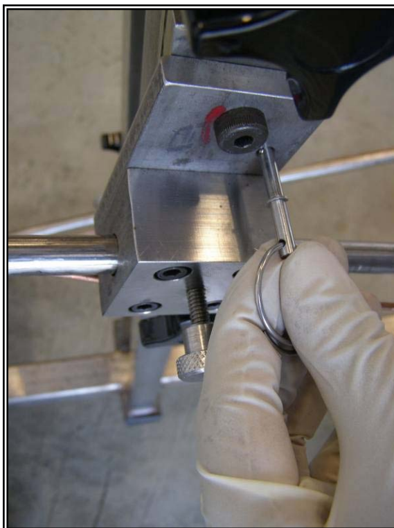
Figure 26. Step 22 Remove pivot point pin.
