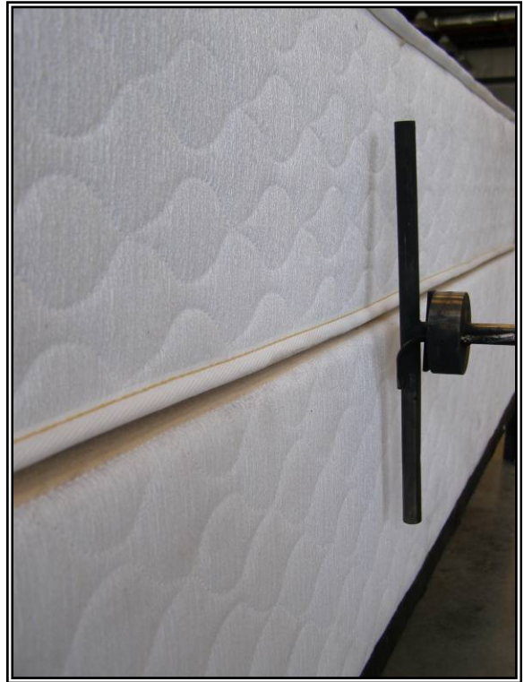
Figure 21. Step 19.a Mattress-foundation alignment.
