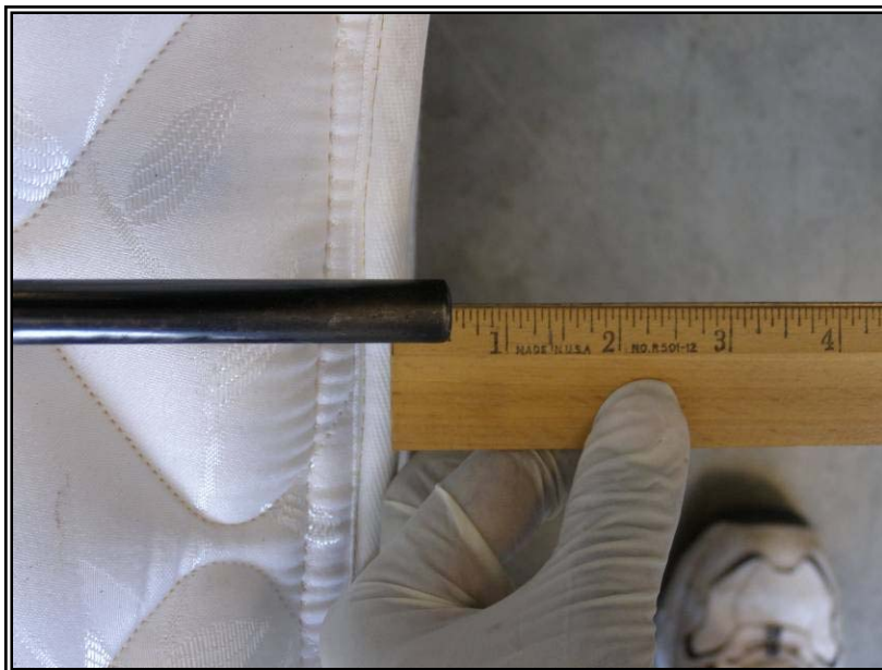
Figure 29. Step 26 Final placement of top burner.
