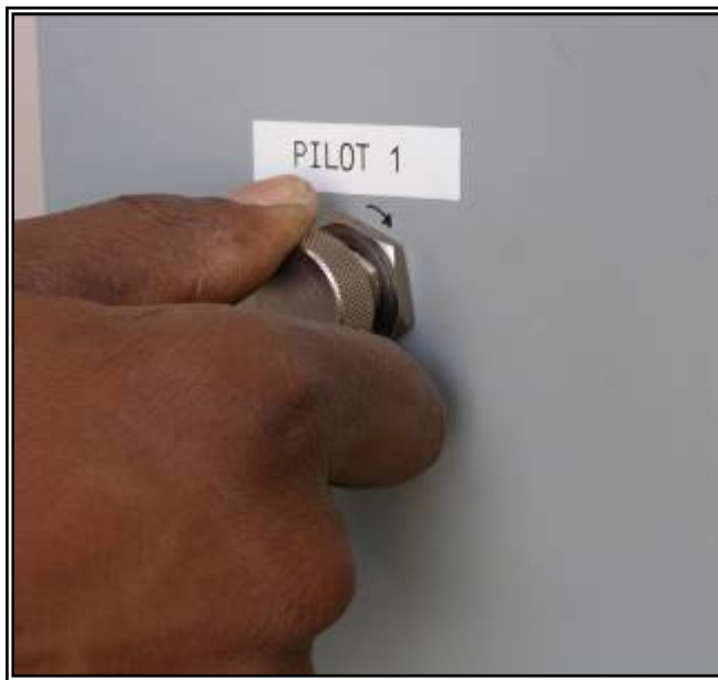
Figure 12. Step 10 Set pilot flow.
