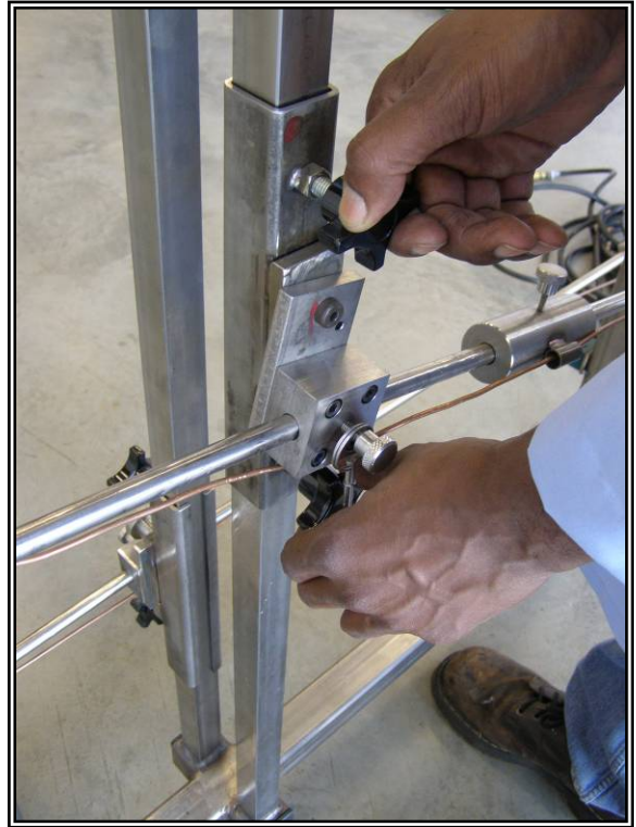
Figure 17. Step 13 Adjust top burner height.
