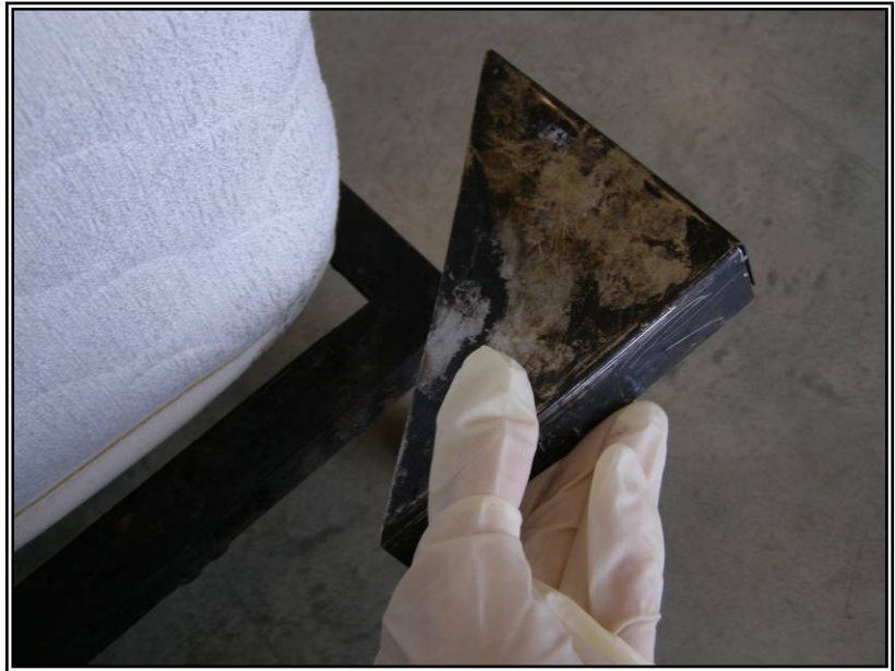
Figure 13. Step 4.c Close open spaces between the test frame and specimen.
