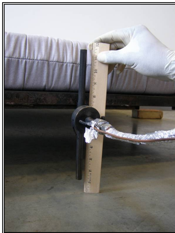
Figure 37. 16.1 Side burner one inch above test floor.
