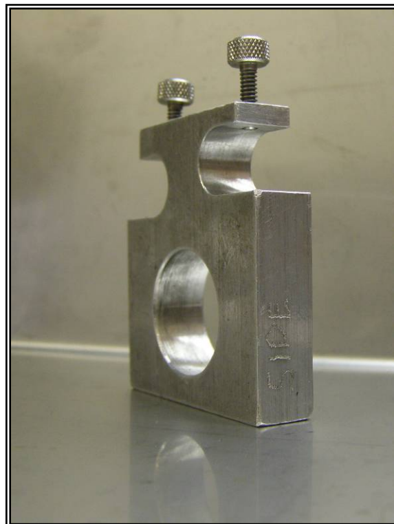
Figure 39. Burner stand-off foot jig
