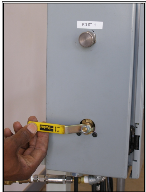
Figure 2. Step 6 Open the ball valves for both burner pilots.
