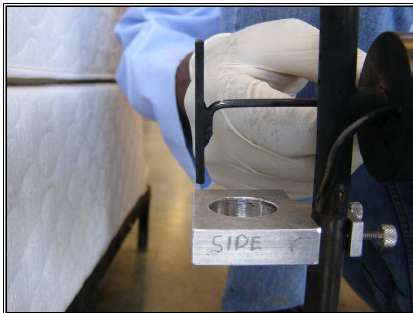
Figure 25. Step 21 Set stand-off foot distance with jig.
