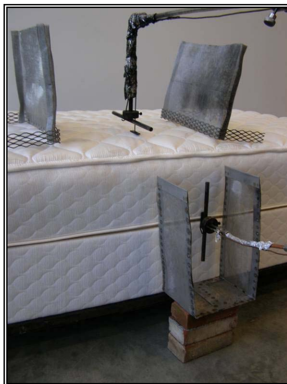
Figure 32. Step 35 Screens placed around burners.
