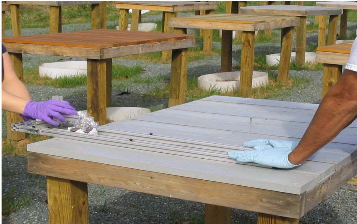
Figure E-2. Sampling to Determine Dislodgeable Arsenic (DAs) Residues on CCA-Treated Wood Using the CPSC Wipe Sampling Apparatus
