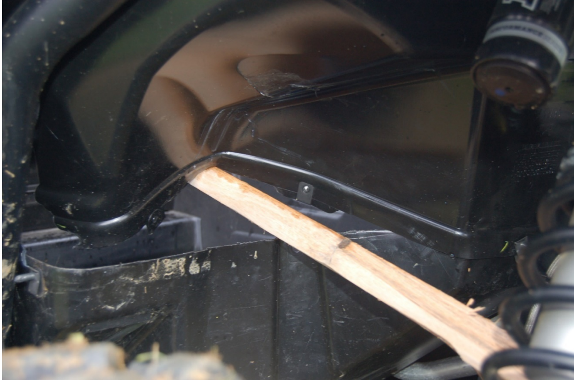
Figure 19: Run 2 External Photo Showing How Stick Passed Between Firewall and Floorboard
