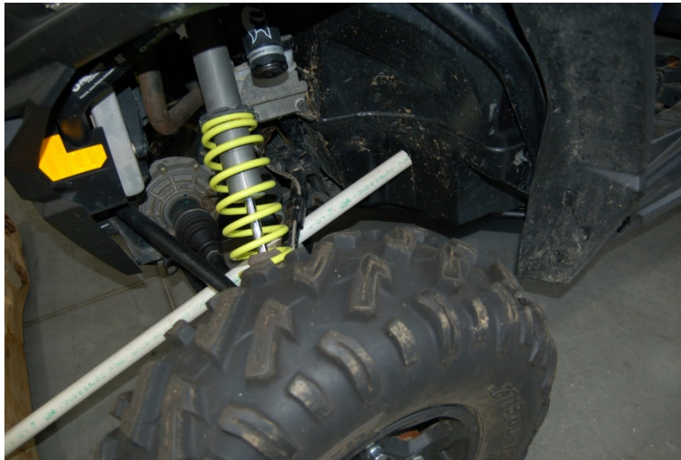
Figure 1: Simulated Stick at an Angle Where it Could Get Caught up in Suspension of Vehicle A.
