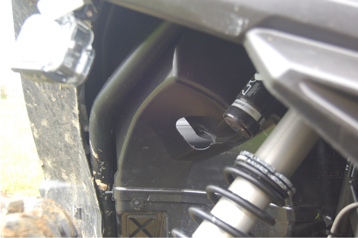
Figure 12: Run 1 Exterior Photo Showing Hole in Firewall Where Stick Penetrated
