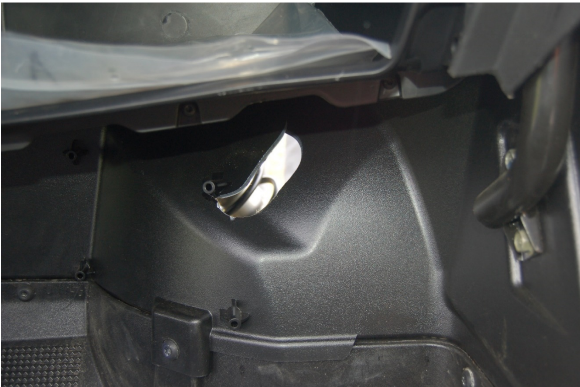
Figure 11: Run 1 Interior Photo Showing Hole in Firewall Where Stick Penetrated
