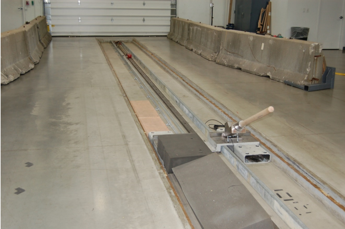
Figure 24: Stick and Stick Holder Mechanism – View Looking Down the Sled Track
