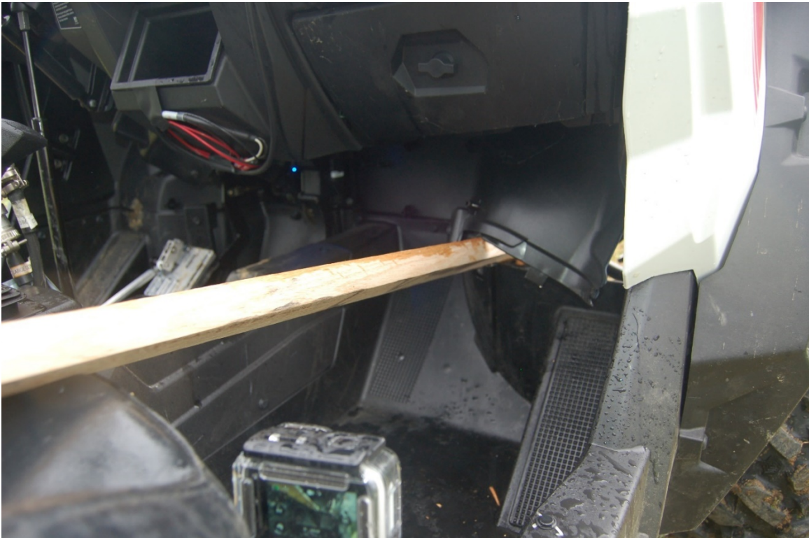
Figure 18: Run 2 Interior Photo Showing How Stick Passed Between Firewall and Floorboard
