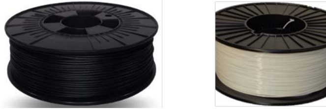
Figure 3: Images of the different filaments used in this study: MWCNT ABS (left) and neat ABS (right).
