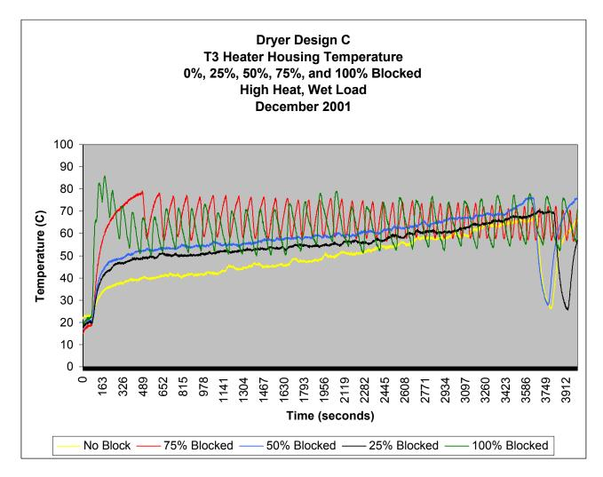
Figure 30. Dryer Design C – T3 Heater Housing Comparison
