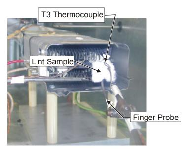
Figure 63. Lint Sample at Heater Intake
