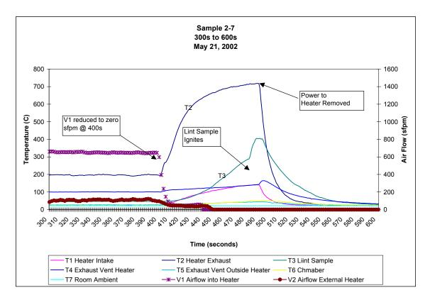
Figure 59. Sample s2-7 Thermocouple Traces
