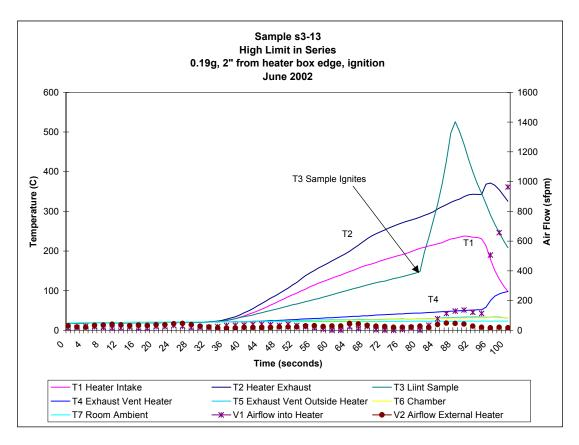
Figure 99. Sample s3-13 Test with the High Limit Thermostat in Series
