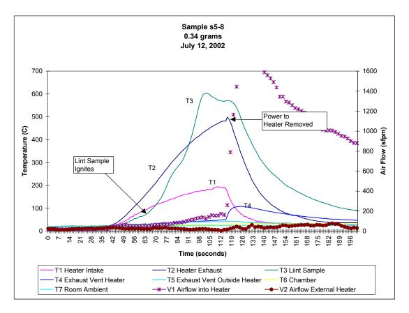
Figure 57. Thermocouple Data for Sample s5-8
