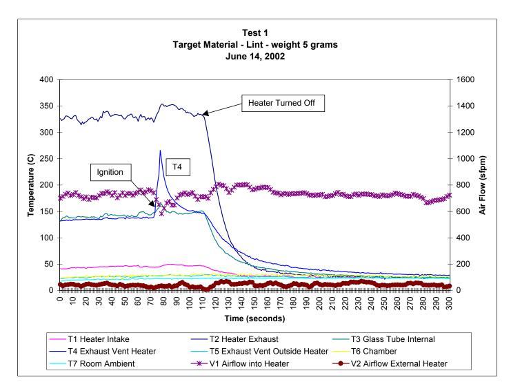
Figure 70. Test 1 – Thermocouple and Airflow Measurements Task 4- Test 1 (Ignition of Target Materials by Exhaust Embers)
