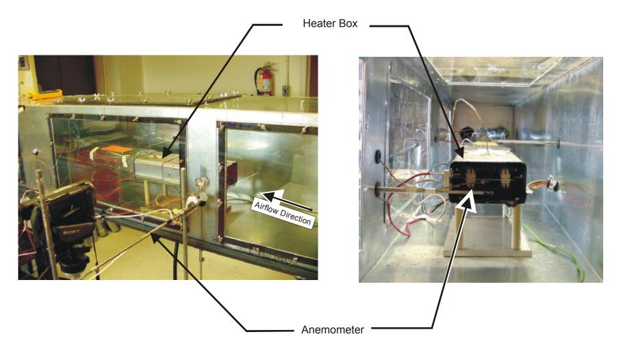
Figure 52. Test Setup for Lint Ignition
