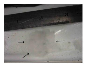
Figure 47. Lint Accumulated at Bottom of Dryer After 100 cycles
