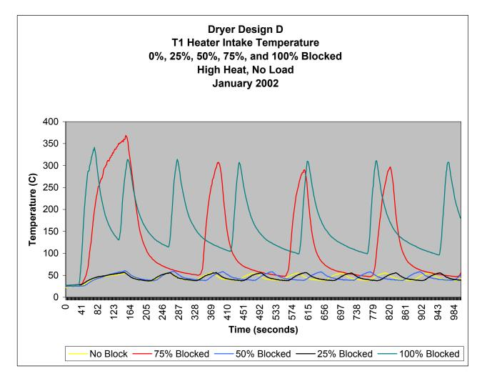
Figure 40. Dryer Design D – T1 Heater Intake Comparison
