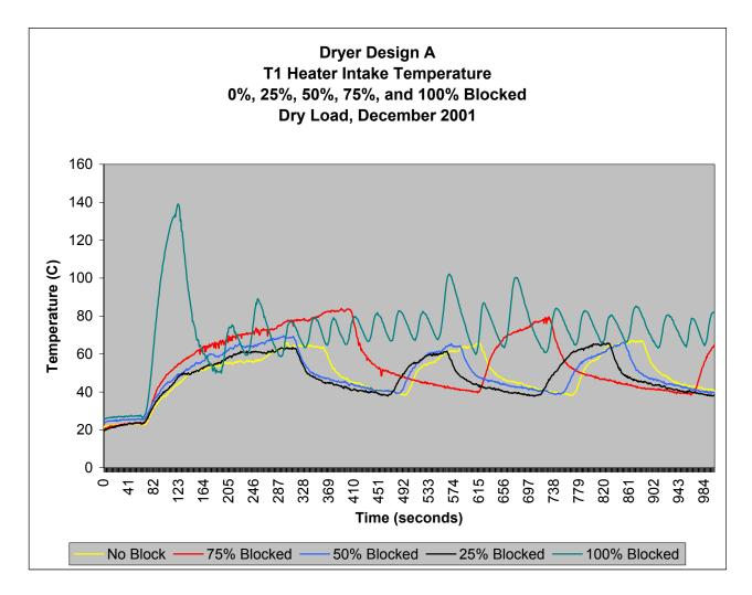
Figure 10. Dryer Design A – T1 Heater Intake Comparison
