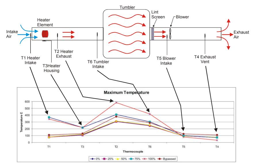
Figure 82. Maximum Temperatures for All Dryers at Each Location and Condition
