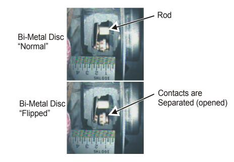
Figure 109. New High Limit Thermostat
