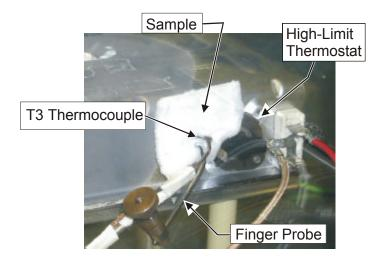
Figure 60. Sample s2-2 Tested at Location D
