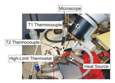
Figure 108. Setup for Testing High-Limit Thermostats
