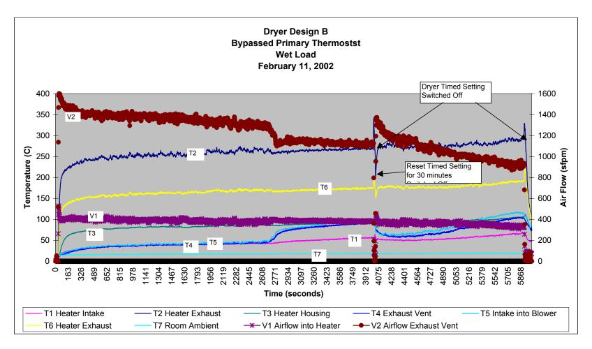
Figure 26. Dryer Design B – Primary Thermostat Bypassed
