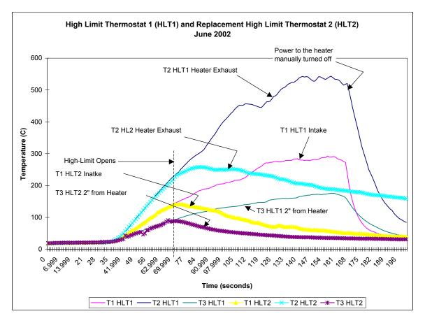
Figure 100. Failed Thermostat compared to a Replacement Thermostat
