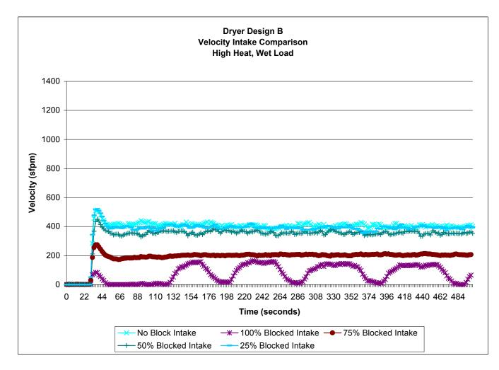
Figure 23. Dryer Design B – Intake Air Velocity
