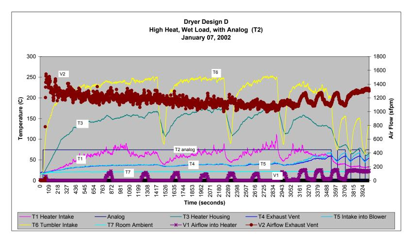
Figure 39. Thermocouple, Airflow and Relay (T2 Analog) Measurements
