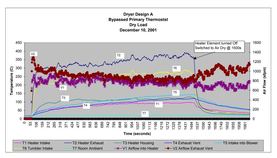
Figure 17. Dryer Design A – Primary Thermostat Bypassed
