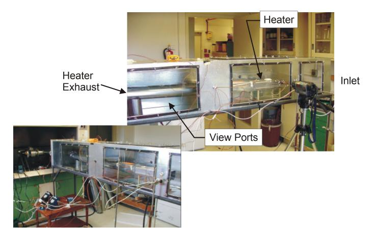
Figure 51. Test Setup for Lint Ignition
