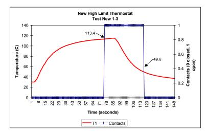
Figure 110. Thermocouple Data for the New High-Limit Thermostat
