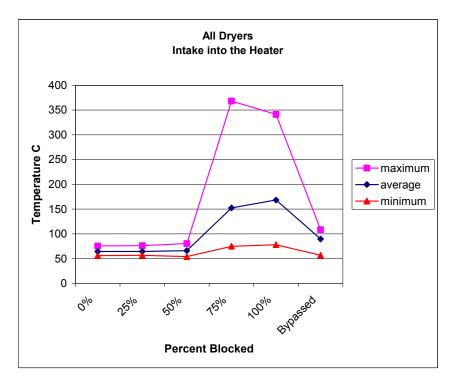
Figure 76. Intake into the Heater
