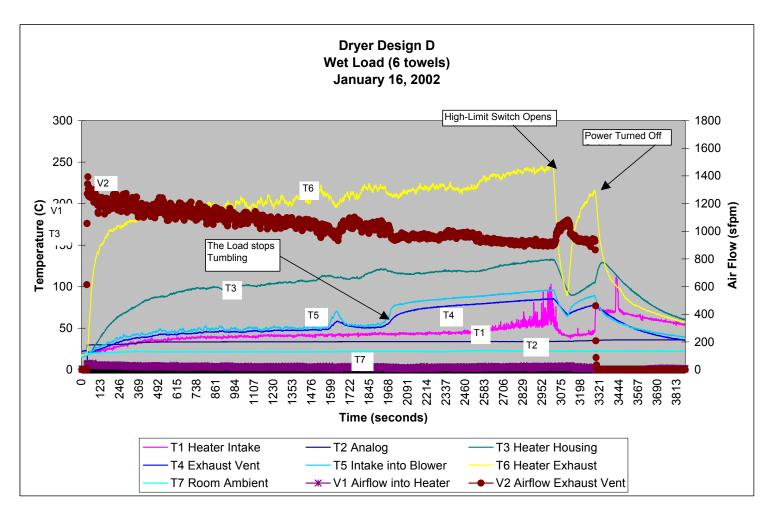
Figure 45. Dryer Design D – Primary Thermostat Bypassed
