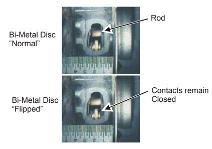
Figure 111. Second Failed High Limit Thermostat, HLT2
