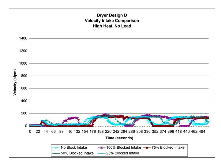
Figure 42. Dryer Design D – Intake Air Velocity
