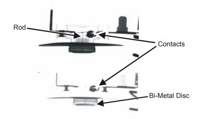
Figure 106. X-ray Images of High-Limit Thermostat 2 (HLT2)
