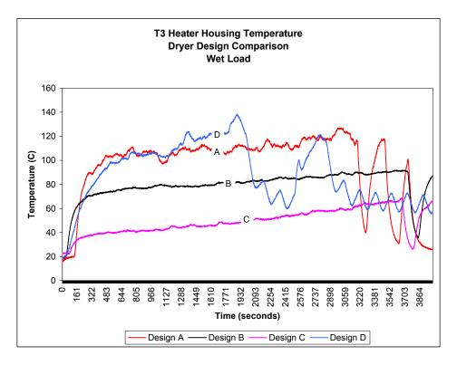
Figure 72. Dryer Design Comparison for T3, Heater Housing
