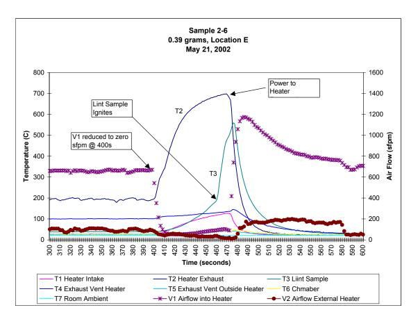
Figure 62. Thermocouple Traces for Sample s2-6 at Location E
