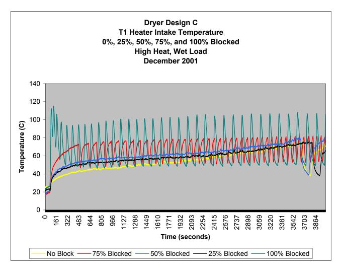
Figure 29. Dryer Design C – T1 Heater Intake Comparison
