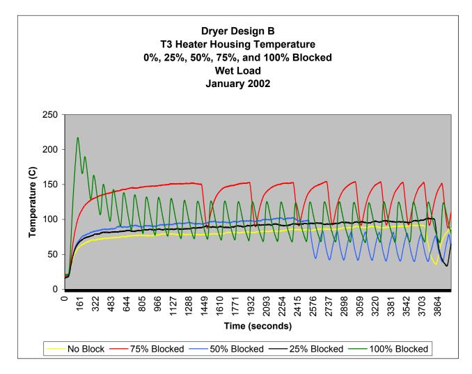
Figure 21. Dryer Design B – T3 Heater Housing Comparison
