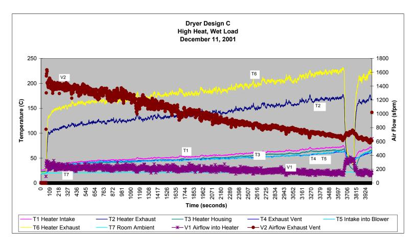
Figure 28. Dryer Design C – Thermocouple and Airflow Measurements (Wet Load)
