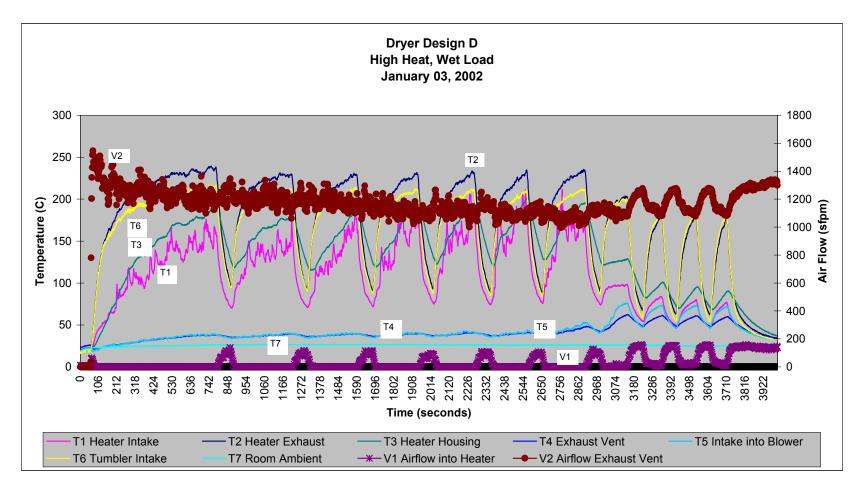
Figure 38. Dryer Design D – Thermocouple and Airflow Measurements (Wet Load)
