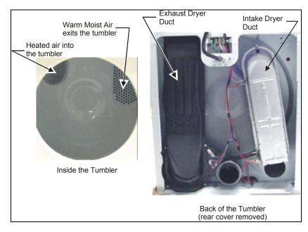
Figure 8. Dryer Design A Intake and Exhaust
