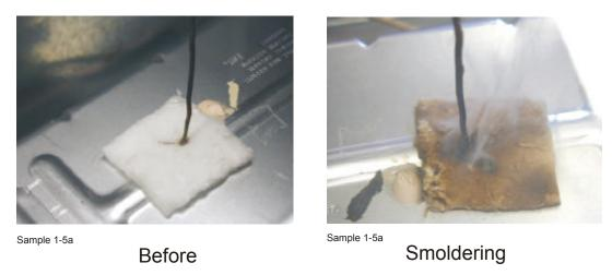
Figure 55. Sample Smoldering at Location A
