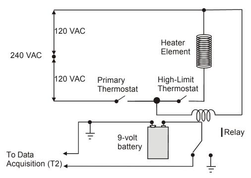
Figure 37. Setup with a Relay and Battery for T2 Analog
