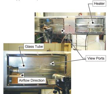
Figure 67. Setup with Glass Tube
