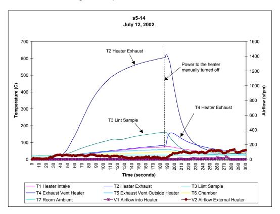
Figure 104. Sample s5-14 with High Limit Thermostat in Series
