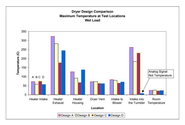
Figure 75. Maximum Temperatures Measured at Location
