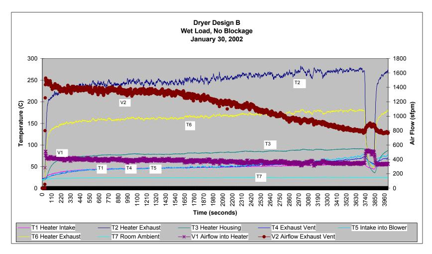
Figure 19. Dryer Design B – Thermocouple and Airflow Measurements (Wet Load)
