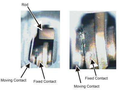
Figure 107. Internal View for High-Limit Thermostat 2
