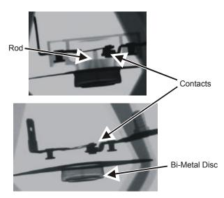
Figure 101. X-ray Images of High-Limit Thermostat 1 (HLT1)
