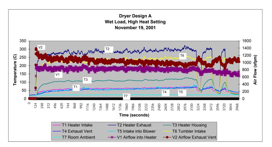
Figure 9. Dryer Design A – Thermocouple and Airflow Measurements with a Wet Load
