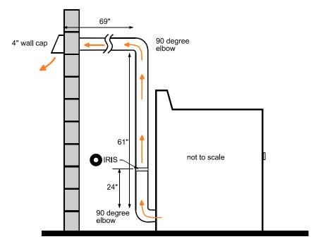
Figure 4. Exhaust Vent Setup
