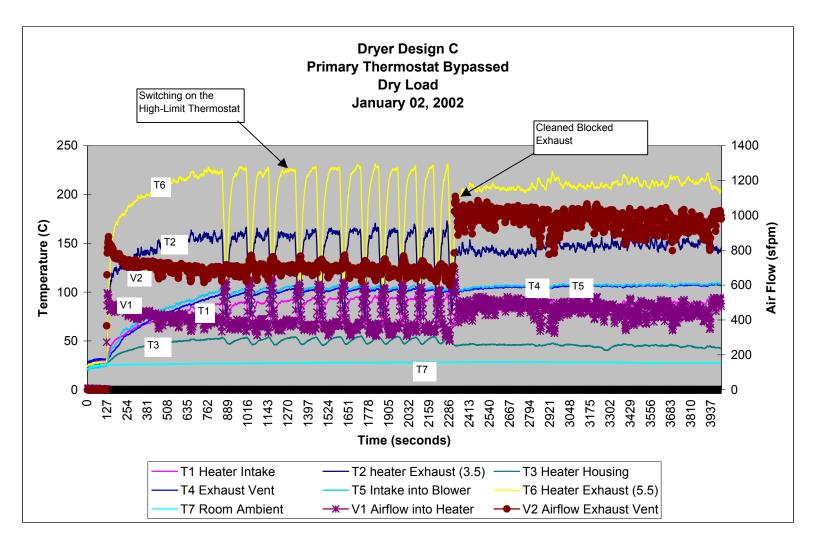
Figure 35. Dryer Design C – Primary Thermostat Bypassed
