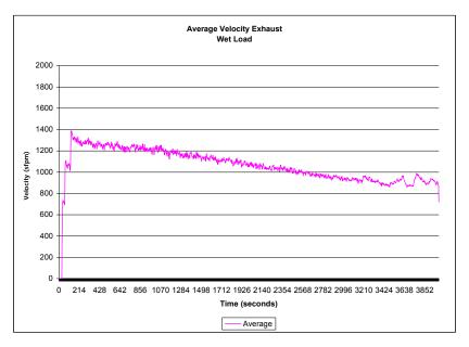
Figure 84. Calculated Average Exhaust Air Velocity
