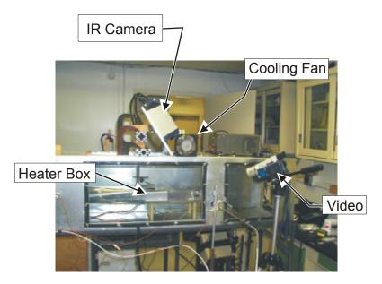
Figure 64. Infrared Camera Setup
