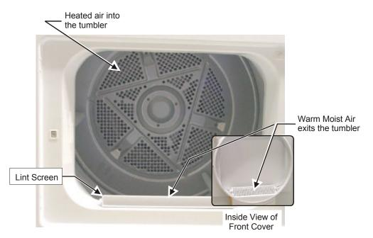
Figure 36. Dryer Design D – Airflow Through the Tumbler
