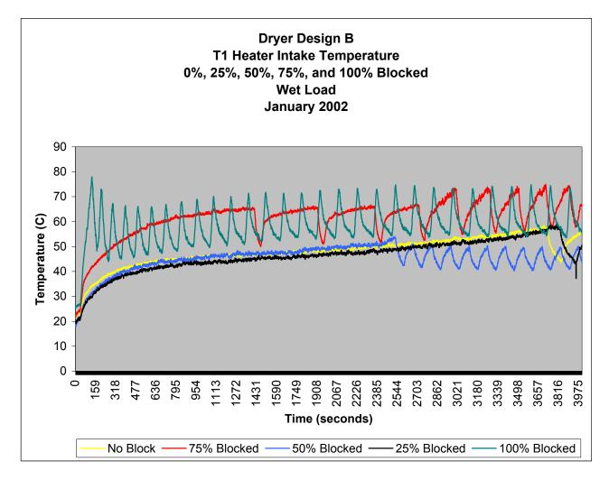
Figure 20. Dryer Design B – T1 Heater Intake Comparison
