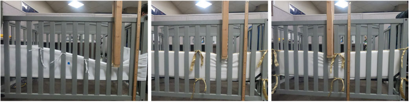
Figure 28: Testing photos of the least deformed products (S06 between attachments, and S20 in two locations).
