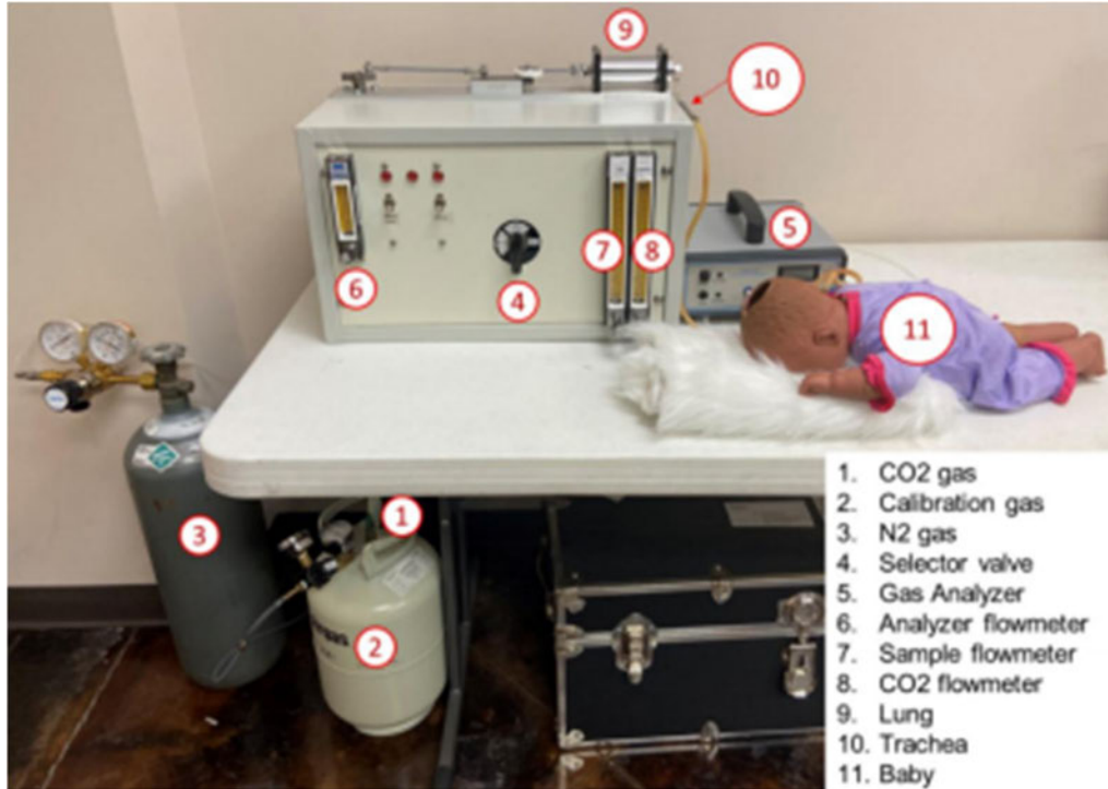
Figure 17: Current CO 2 rebreathing testing setup.
