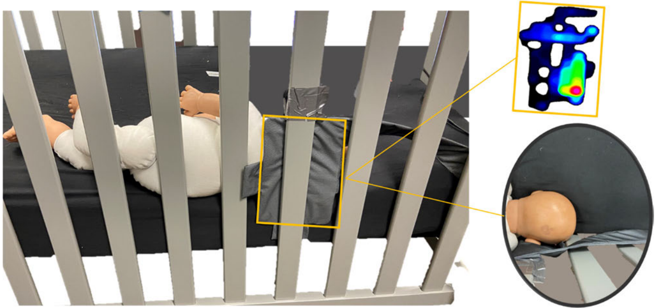
Figure 35: (Left) Simulated crib entrapment/wedging setup, and (Top Right) pressure distribution characteristics.
