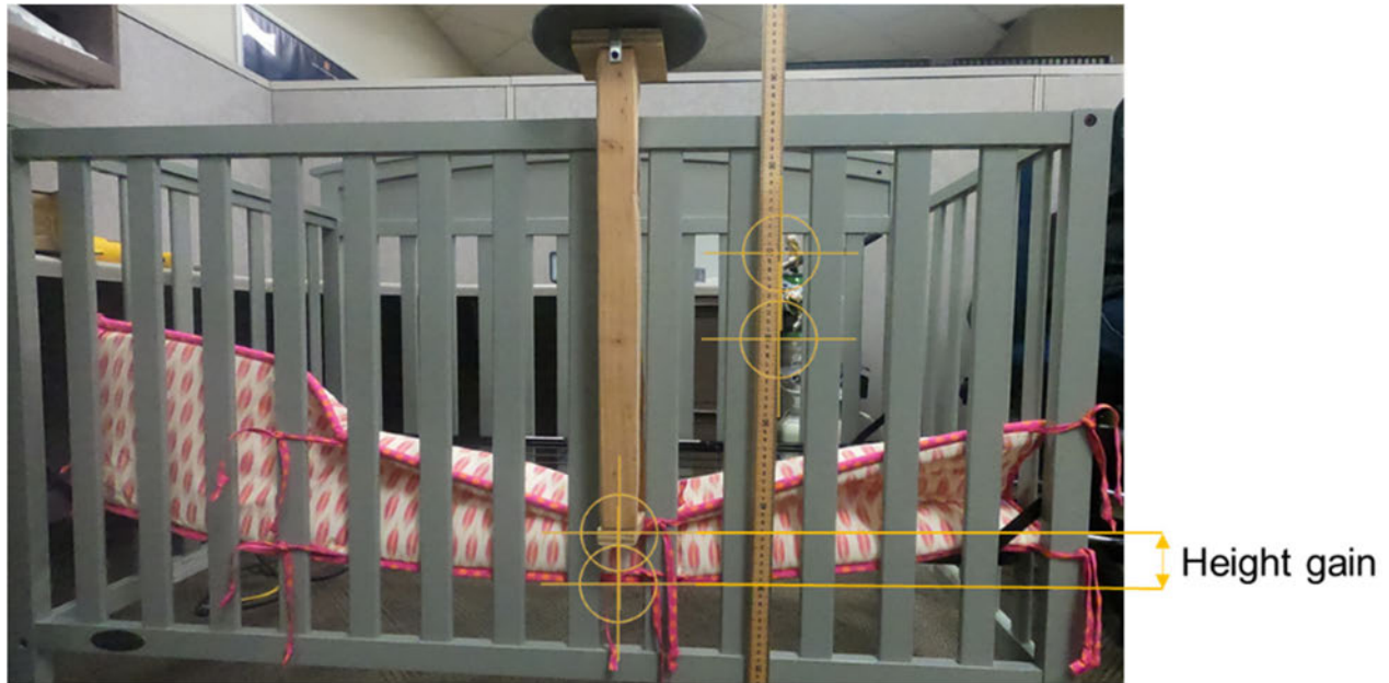
Figure 26: Demonstration of testing protocol, and MATLAB Image Analysis schematic for bumper deformation testing using 9-month-old equivalent load.
