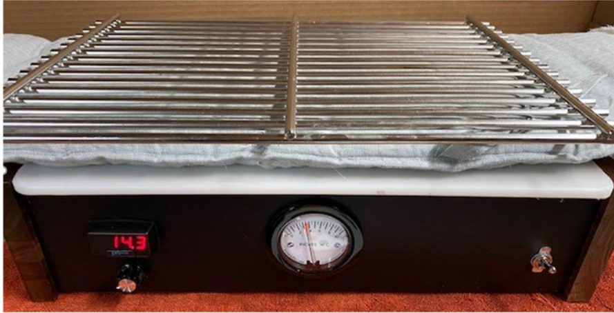
Figure 37: Thermal rebreathing analyzer with sample in place. Here we used a perforated (grate) platform, but we can explore an unperforated (solid) platform in the future.
