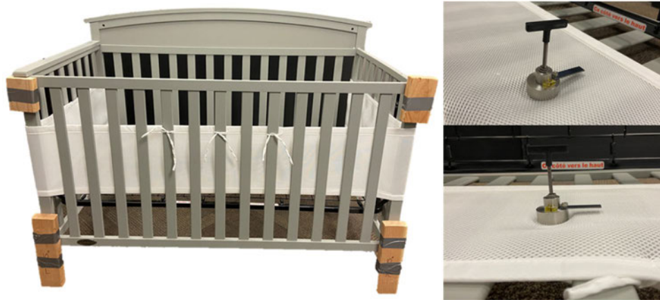
Figure 7: (Left) Crib elevation setup, and (Right) modified firmness fixture placements between slats on rotated crib side.
