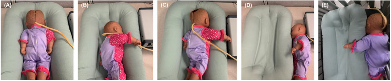
Figure 19: Rebreathing testing scenarios for lounger products. (A) Facedown. (B) Facing the side from inside. (C) Inside corner. (D) Facing the side from outside. (E) Intersection between sample and mattress.
