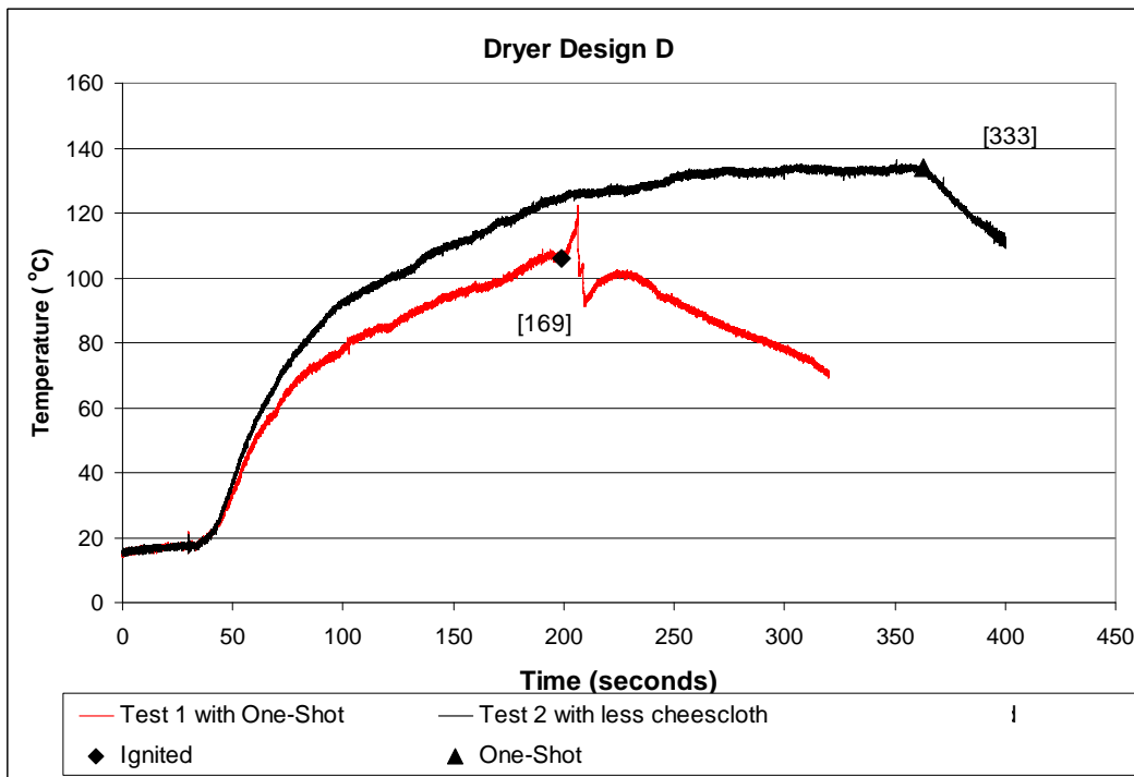
Times in [ ] are from the video and represent elapsed time from when the clothes dryer was started. The x-axis time scale represents the elapsed time when the data acquisition system was started.
