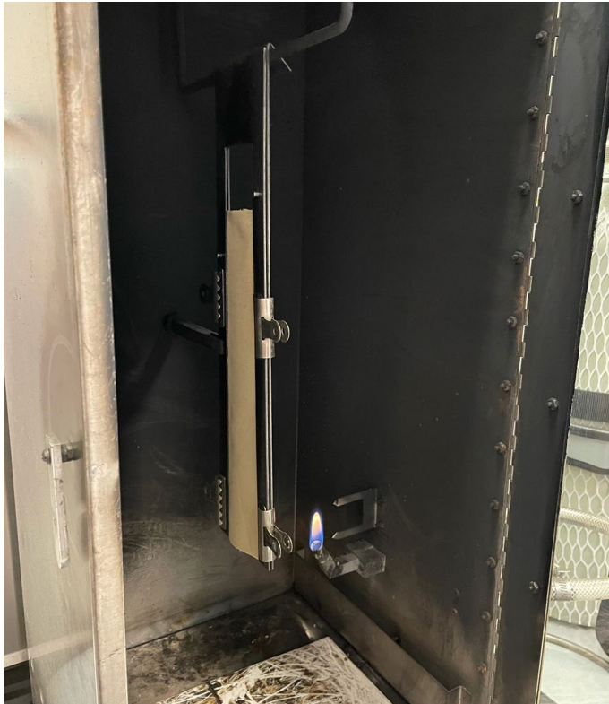
Figure 2: CGSB-182.1 test set up
