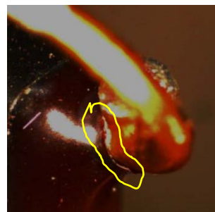
Solder in the cracks of the epoxy/electrode
