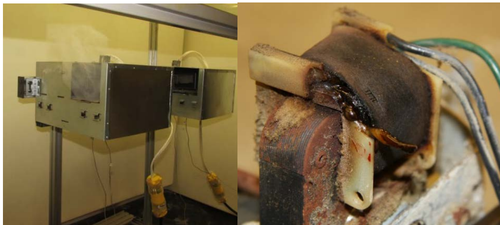
Figure 27. Sub 41 Test Group 3 - Lock-Rotor Test producing smoke and post examination
