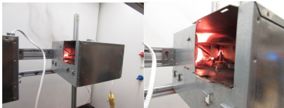
Figure 19. Bypassed TCO lock-rotor test
