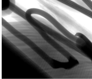
Sub 10 - After conditioning @ 105°C 64.5 hours
