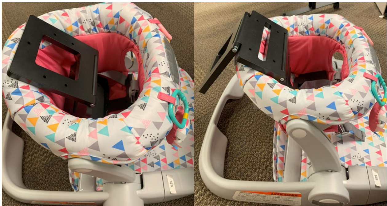
Figure 246. Example of the five-segment sagittal plane device not performing well in an upright infant floor seat product.
