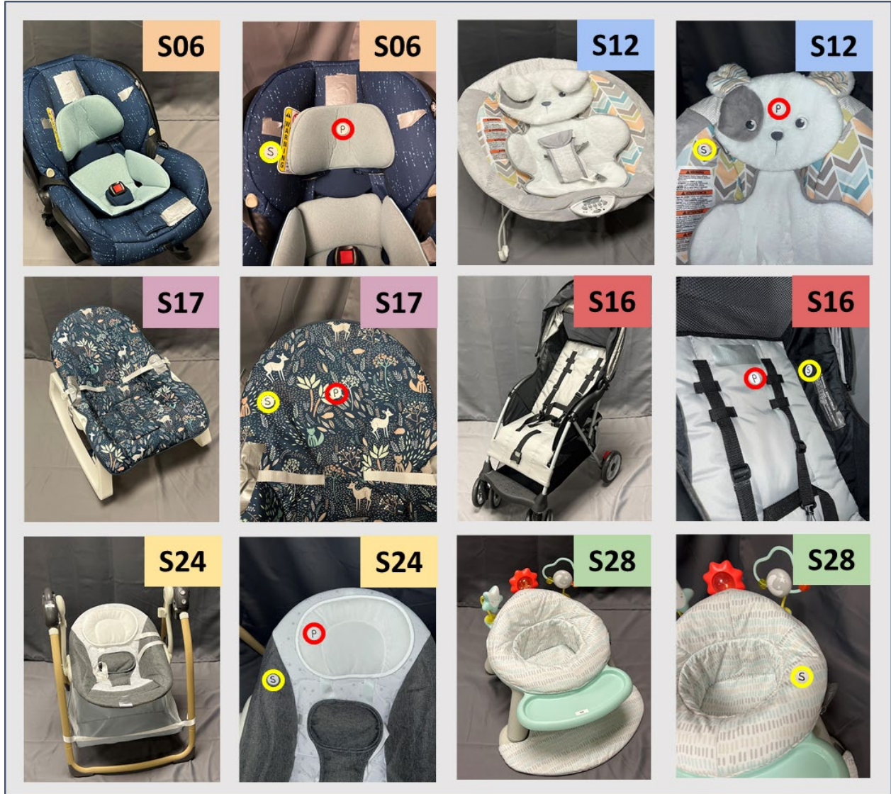
Figure 30. Photos showing the prone (P, red circles) and first contact supine (S, yellow circles) locations for firmness and airflow testing on a representative seated product from each product category.
