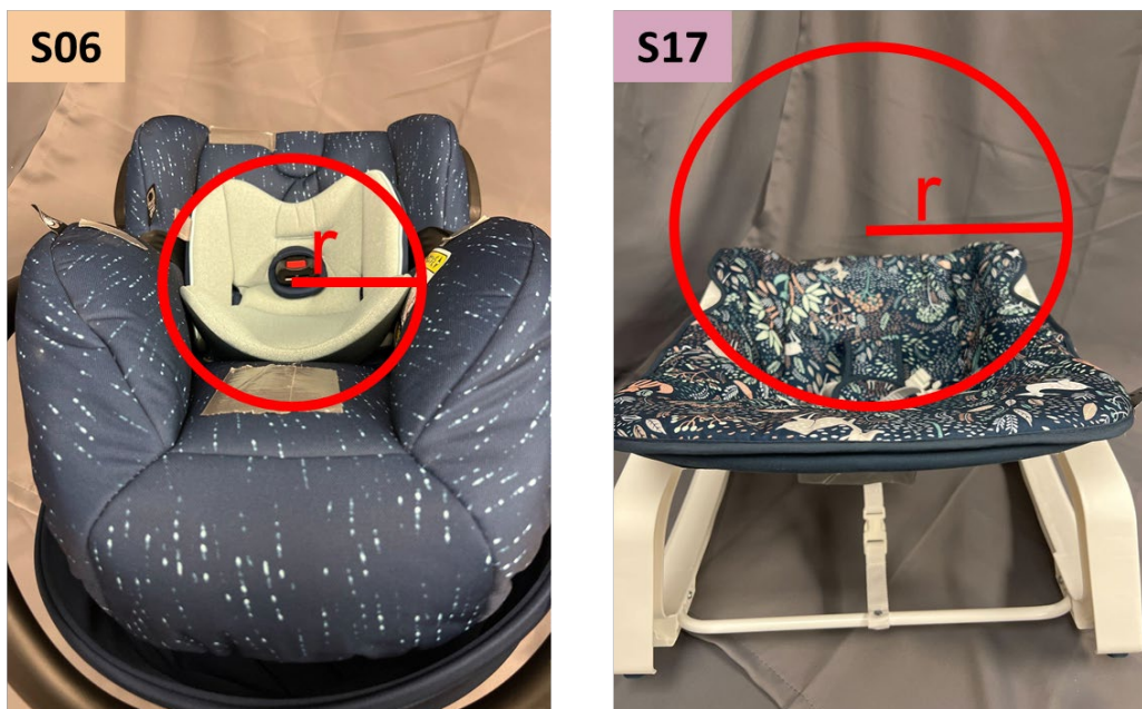
Figure 21. Example of the best-fit circle and the radius (r) for two different products, showing how the smaller radius correlates to a more concave product.
