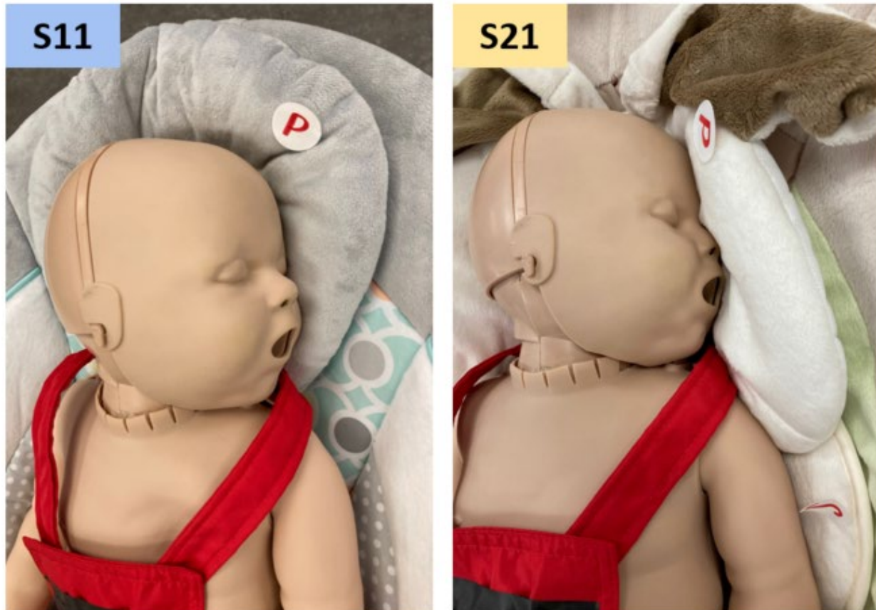
Figure 27. Depiction of a smaller pillow in S11 resulting in no mouth/nose contact during supine lying with a head turn, compared to a larger pillow in S21 which results in mouth/nose contact.
