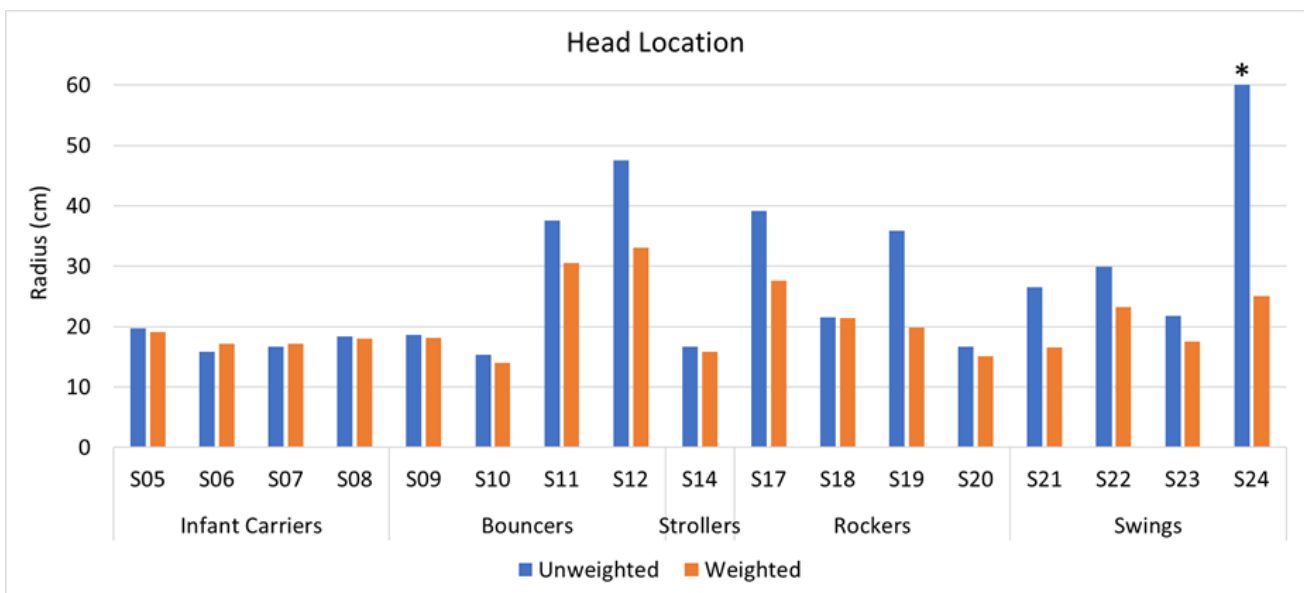
Figure 22. The concavity of each product at the head location, with (weighted) and without (unweighted) the infant five-segment sagittal plane device in the intended position. The smaller the radius, the more concave the product. The S24 unweighted radius was 128 cm.
