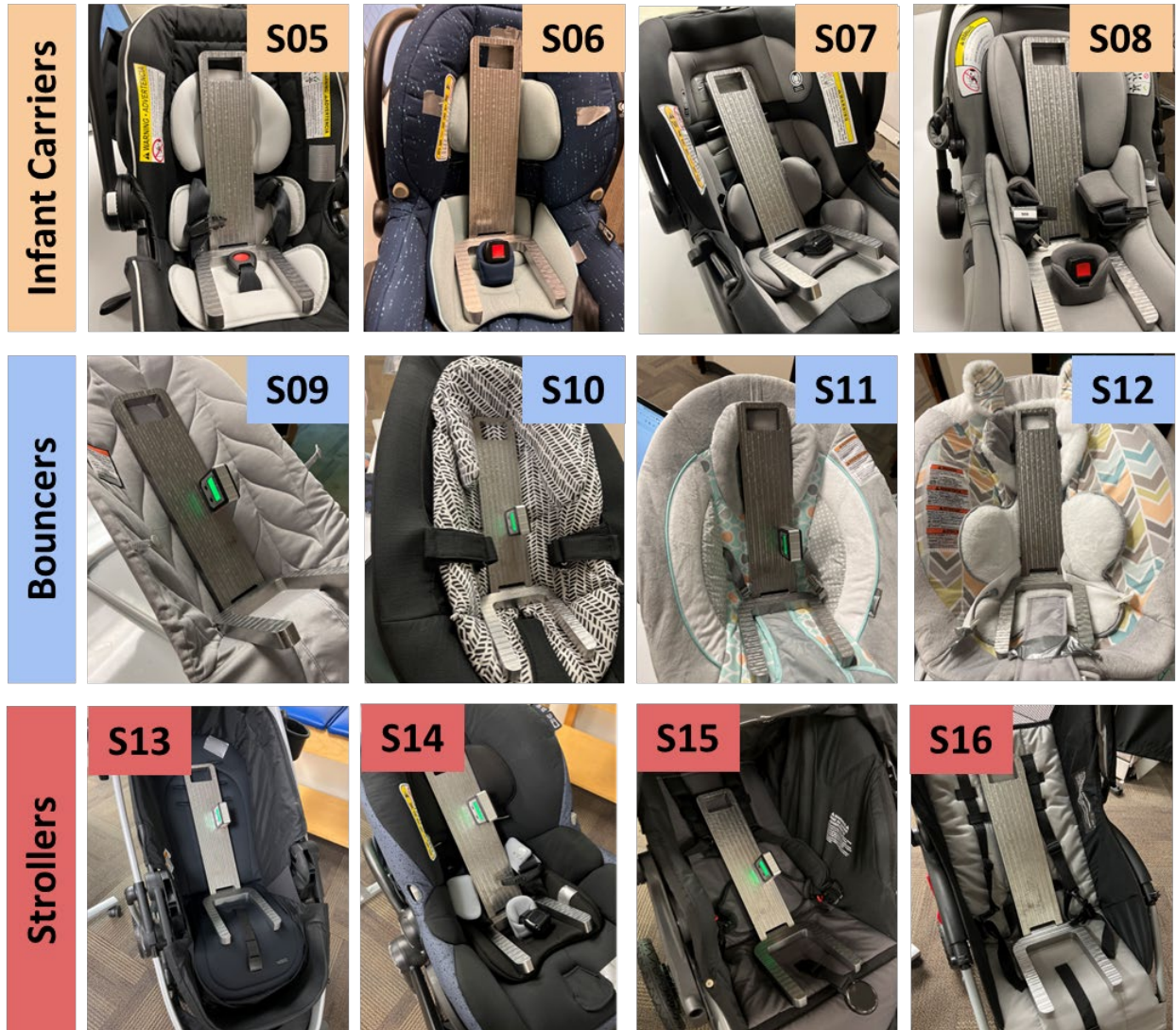
Figure 8. Photos of testing with the infant-sized hinged weight gauge for infant carriers, bouncers, and strollers.
