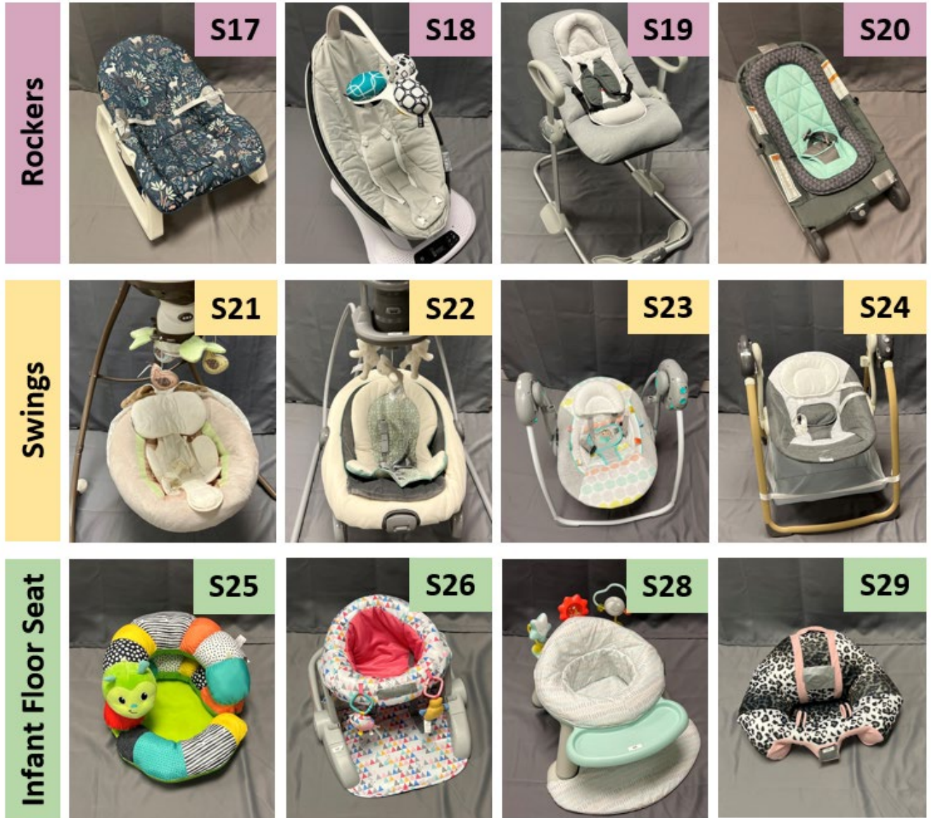
Figure 6. Photos of the rockers, swings, and infant floor seats chosen for this study along with the sample numbers.
