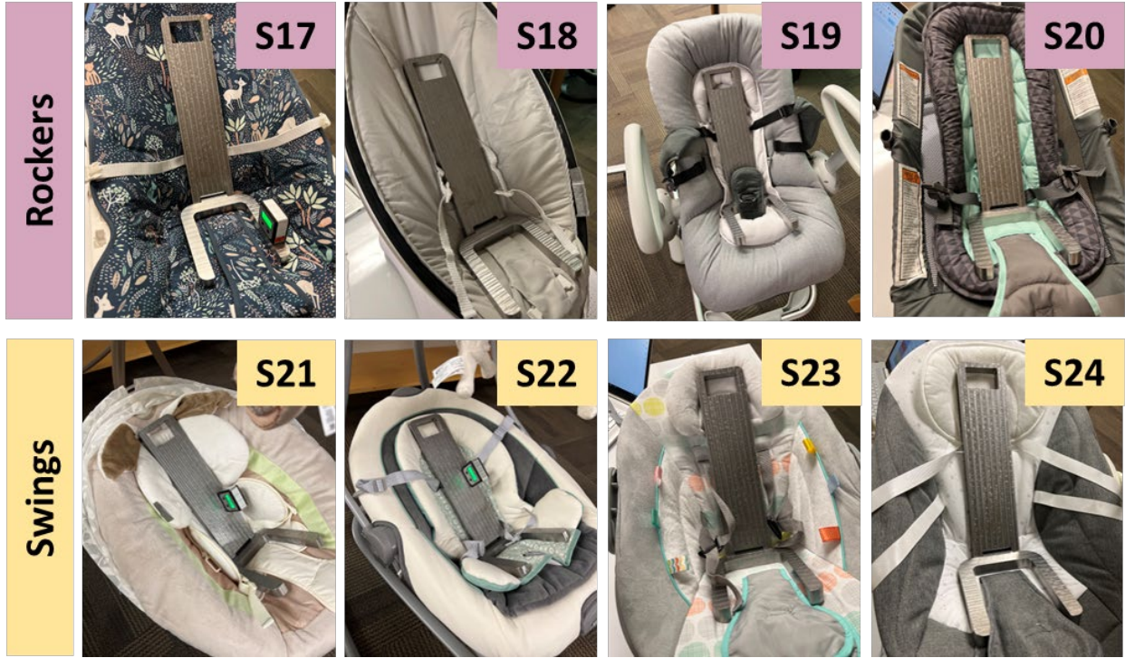
Figure 9. Photos of testing with the infant-sized hinged weight gauge for rockers and swings.
