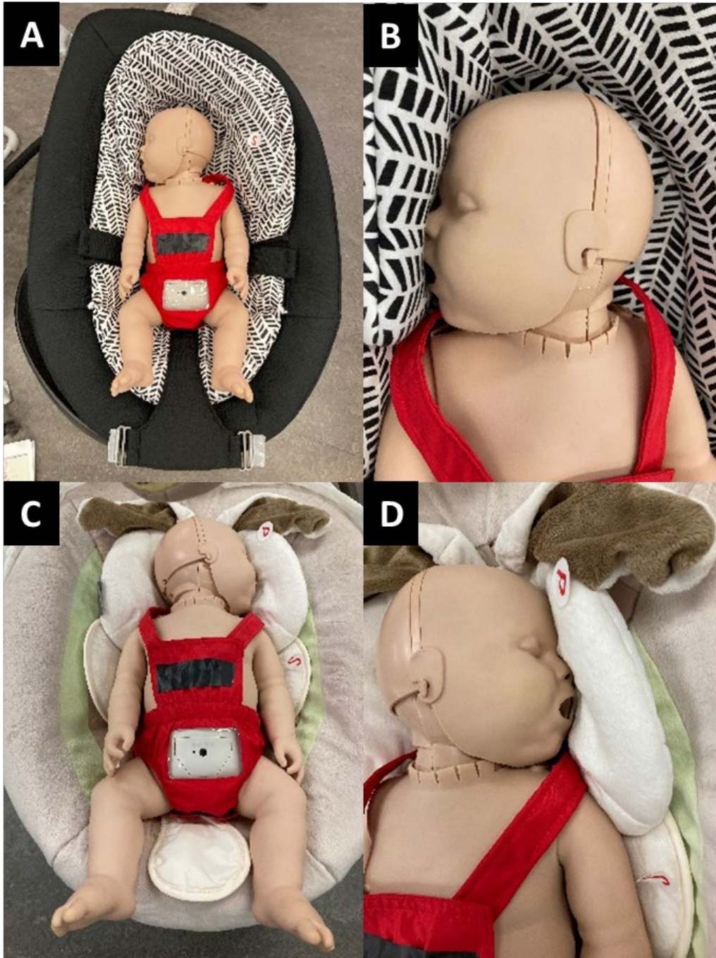
Figure 17. Head rotation failures for (A) and (B) product S10 in the intended position; and (C) and (D) product S21 in the slouched position. Product S10 failed in the intended position, while product S21 failed in both the intended and the slouched position.
